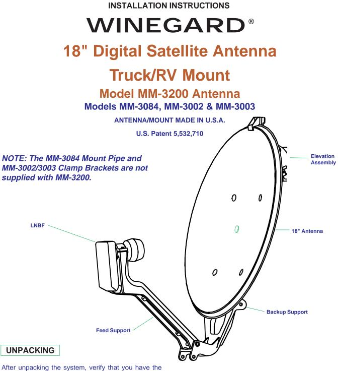
After unpacking the system, verify that you have the following: antenna/mount, elevation assembly, feed support w/LNBF & coaxial cable attached, compass and storage bag. If you do not, call Winegard Company at 1-800-288-8094 between the hours of 8:00 a.m. and 3:30 p.m central time, Monday through Friday.
